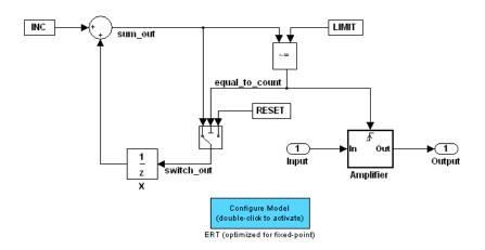
**6** You can set up the Configuration Wizard block to invoke the build process after executing its configuration script. If you do not want to use this feature, skip to the next step.
