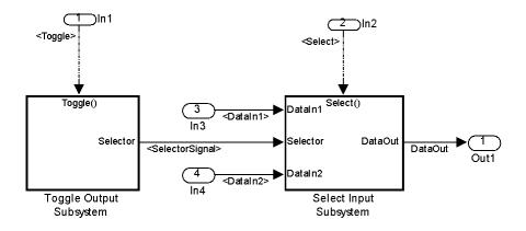
In the preceding model, the Stateflow chart can assert either of two scalar signals, Toggle and Select.
