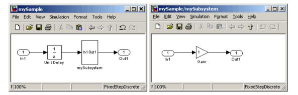
Assume that the subsystem is atomic, the **Real-Time Workshop system code** is Reusable function, memory sections have been created and assigned as shown in the next two tables, and all data memory sections specify **Pragma surrounds** to be Each variable.
