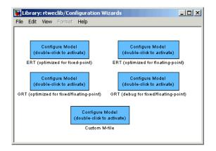
When you add one of the preset Configuration Wizard blocks to your model and double-click it, a predefined M-file script executes and configures all parameters of the model's active configuration set without manual intervention. The preset blocks configure the options optimally for one of the following cases:
