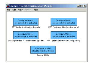
**5** Select the Configuration Wizard block you want to use and drag and drop it into your model. In the figure below, the ERT (optimized for fixed-point) Configuration Wizard block has been added to the model.
